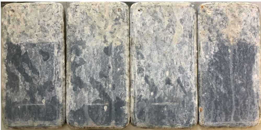
Figure 4. From left to right, Panel 11, 12, 14 and 15 at 4200 hours of cyclical testing (Requirement for CX)
