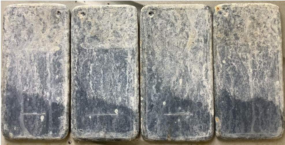
Figure 3. From left to right, Panel 11, 12, 14 and 15 at 2688 hours of cyclical testing (Requirement for C5 Very High)
