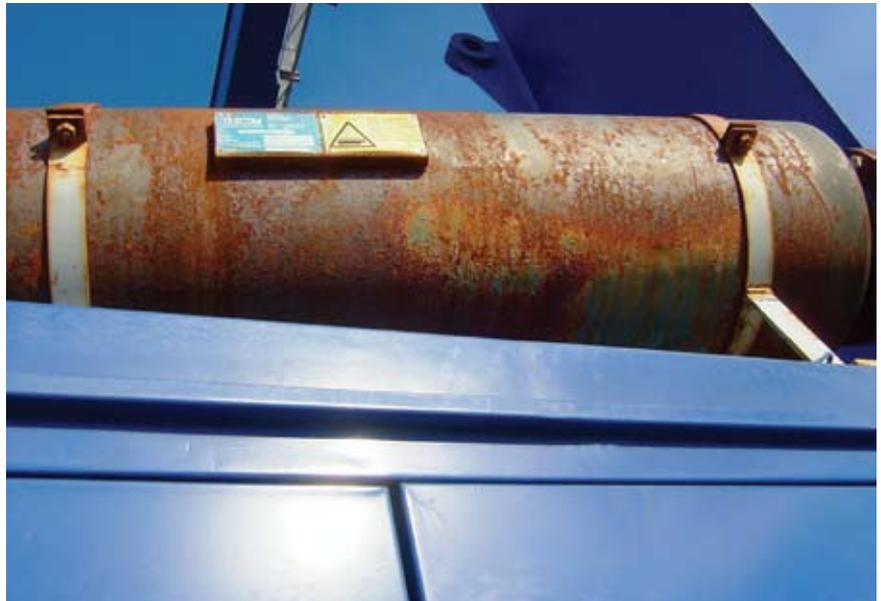
**ABOVE ▲** If flash rust occurs on the steel substrate, the steel should be tested for contamination, because the rust is probably the result of non-visible soluble salt contamination. Without some ionic species present, there will not be rust. Even very low soluble salt levels can cause an appreciable amount of flash rust.
