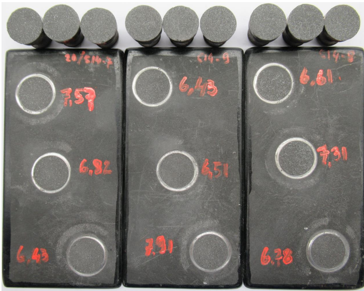
Photo 3: Panels 20/0514-7(5), 20/0514-9(20) and 20/514-8(18!) after 720 hours Water Condensation test
