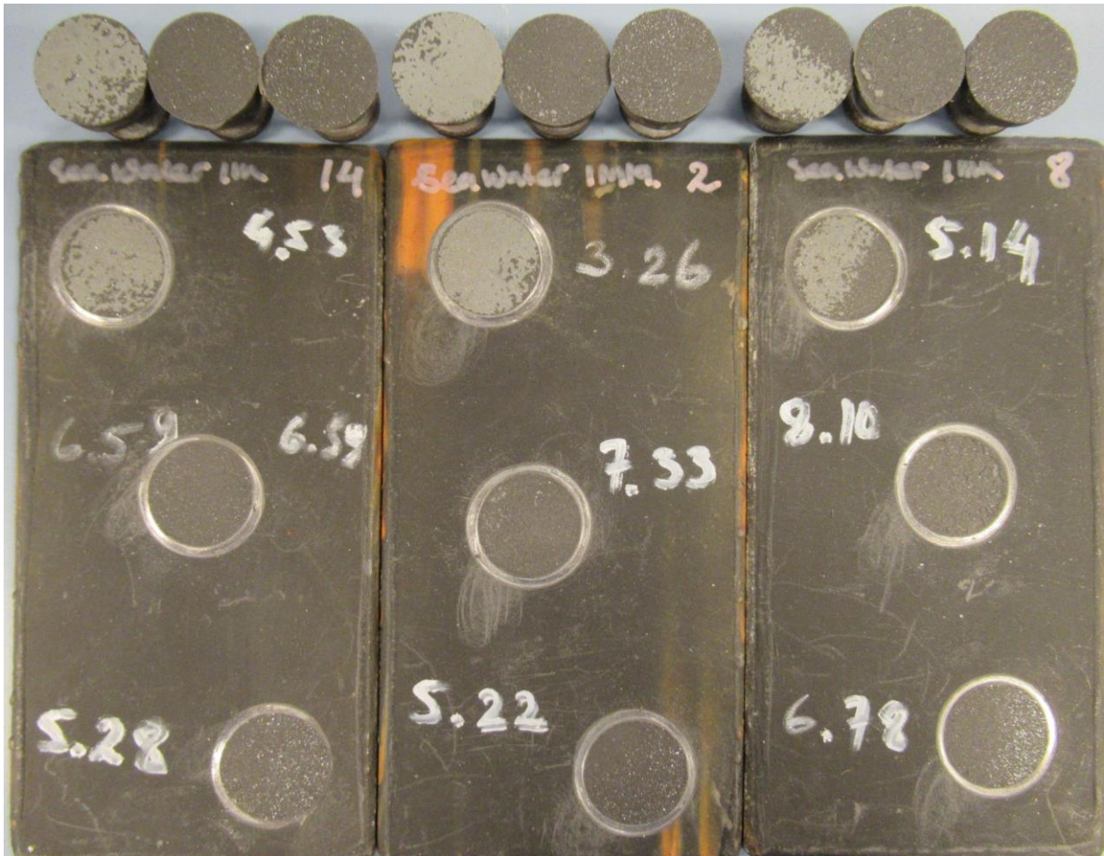
Photo 3: Pull off test panel 20/0514-12(14), 20/0514-10(2) and 20/0514-11(8) after 4000 hours Immersion test.
