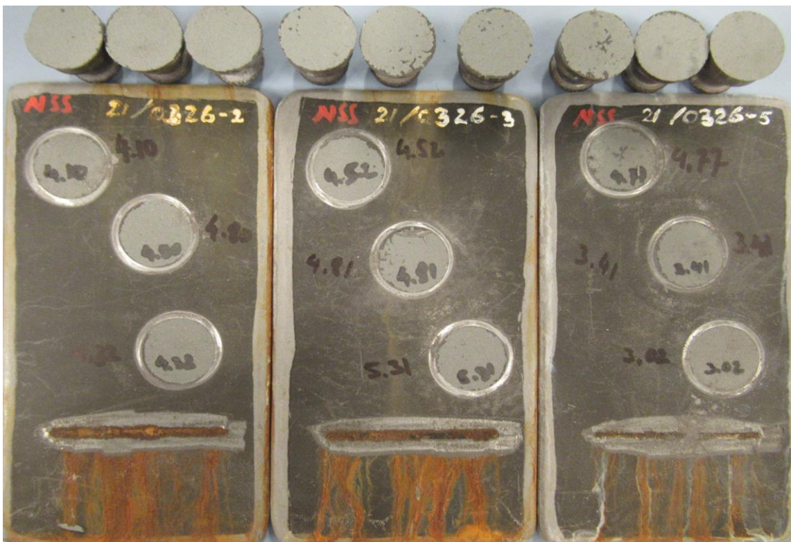
Photo 2a: 21/0326-3, 21/0326-3 and 21/0326-5 after 1440 hours Neutral Salt Spray test
