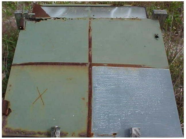
Quad Tests- The Army Truck Door is divided into Quads- Lower Right Quadrant is ZINGA ALONE (PRIMER ALONE); Upper Right Quadrant is ZINGA With CARC top coating. Lower Left Quad is NO ZINGA, only top coat; Upper Left Quad is ZINGA with top coat and CARC: KEY Results: ZINGA ONLY shows NO RUST; the Quad w/o ZINGA shows rust coming thru at several places, showing major rust after 3 years.
