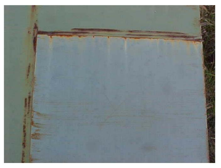
Quad Tests- This is lower right quadrant of Paint A. This is Zinc rich paint A ONLY coating. Note that rust is coming through the paint strokes Clearly A has been Ineffective In rust prevention.
