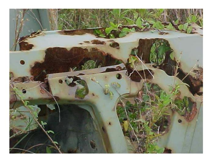
Army trucks after 3 years of exposure using typical epoxy paints. 3 years of sea side exposure shows massive corrosion and complete loss of steel panels and structures
