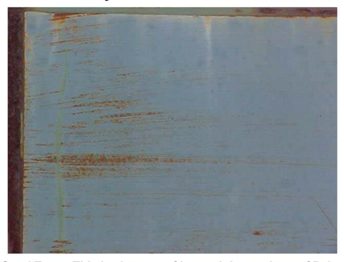
Quad Tests- This is close up of lower right quadrant of Paint A. This is Zinc rich paint A ONLY coating. Note that rust is coming through the paint strokes. Clearly A has been Ineffective In rust prevention. Note also the lack of cathodic reaction, as very little Zinc salts can be seen. Extremely poor cathodic Protection.
