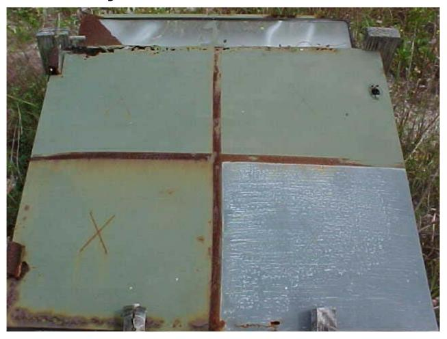
NOTICE the QUAD Dividing lines. This is where NO ZINGA or protection was Provided. Rust has caused major damage in these areas. With no protection the Rust in just 3 years has ruined this door. This door is not serviceable and will have To be replaced.
