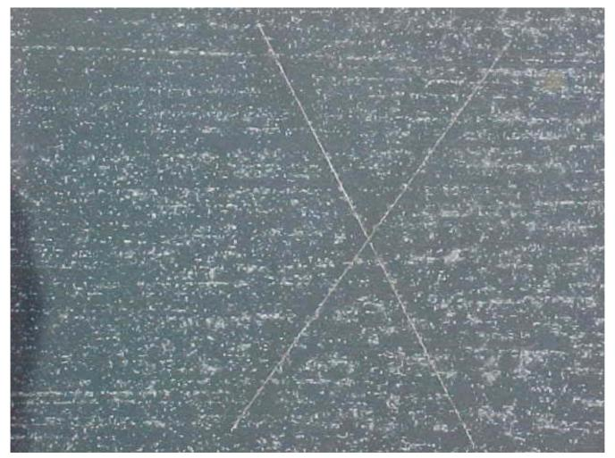
Quad Tests: This shows a CLOSE UP view of the lower right quadrant which was 'coated with ZINGA ONLY. The cathodic reaction can be seen clearly from the Zinc Salts (white-grey) forming on the surface. Note no rust at all even in the CUT. This is a outstanding picture of cathodic protection.
