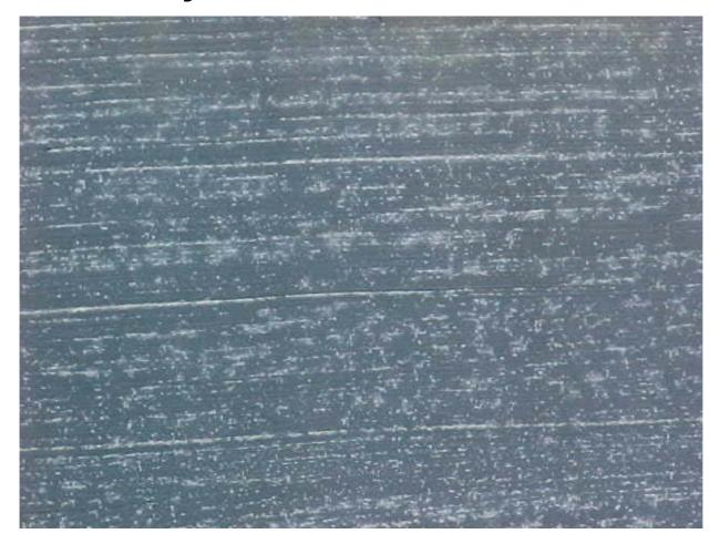
Quad tests- This is a extreme close up of ZINGA ONLY Quadrant showing absolutely NO RUST forming or coming Through due to paint strokes. NO RUST
