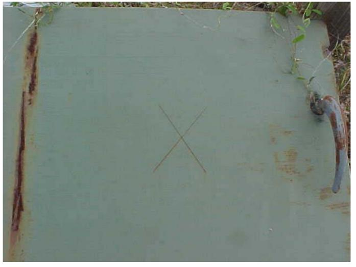
Quad Tests- This is upper right quadrant of Zinc rich paint A. Note that rust is coming through even with the paint A and a top coat. Clearly the Zinc rich paint has been ineffective In rust prevention after just 3 years in sea air environment.
