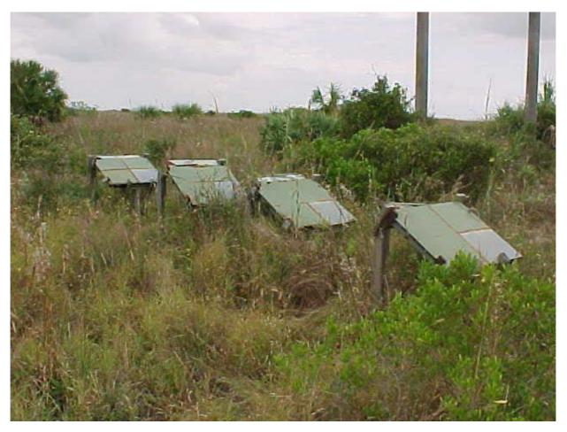
Quad Tests – Doors were divided into quadrants for a test of coatings and primers. Each quadrant was used for primer only; top coat only; & primer and top coats
