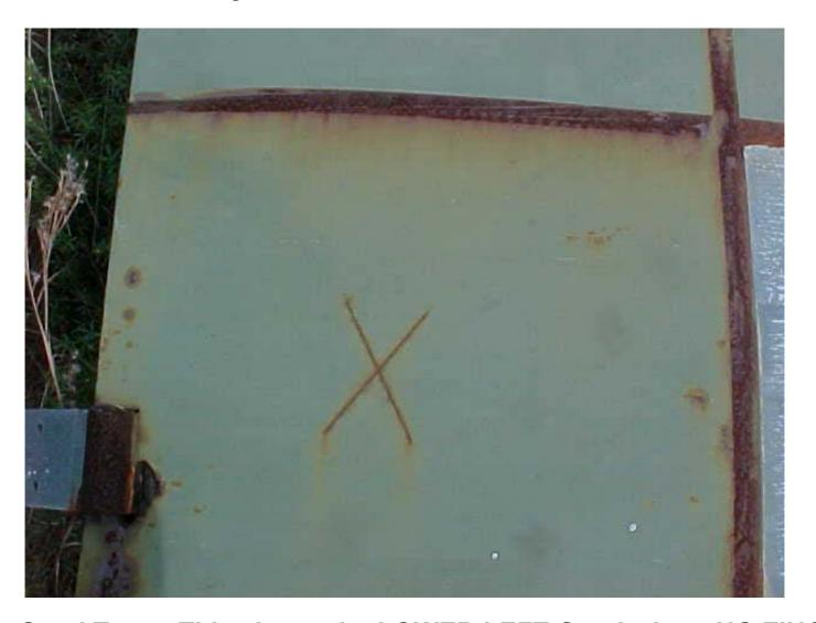
Quad Tests: This shows the LOWER LEFT Quad where NO ZINGA Has been applied – this is top coat only and after 3 years major Rust can be seen coming through all over the door.
