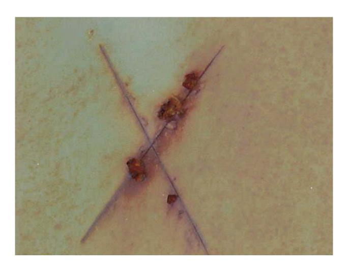
Control Door (epoxy paint)— Close up of "cut" shows deep pitting and the beginning of holes in the steel control door — this is the result of 3 years at the US Army sea side test site.
