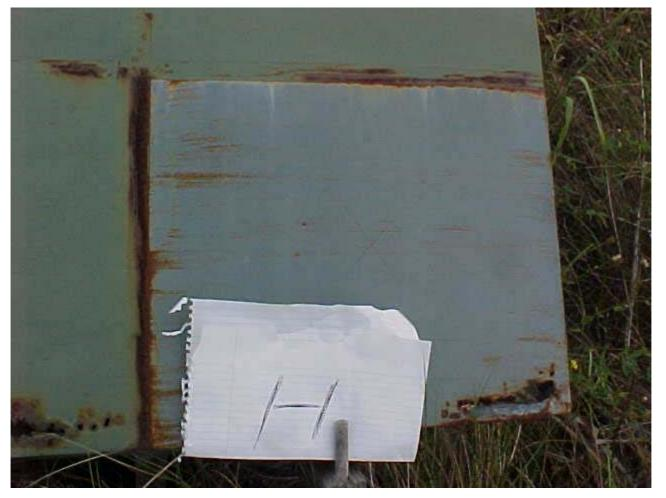
Quad Tests- This is lower right quadrant of Zinc rich paint A. This is Zinc rich paint A ONLY coating. Note that rust is coming through the paint strokes .Clearly the A has been Ineffective In rust prevention. Note also the lack of cathodic reaction, as very little Zinc salts can be seen. Extremely poor cathodic Protection.
