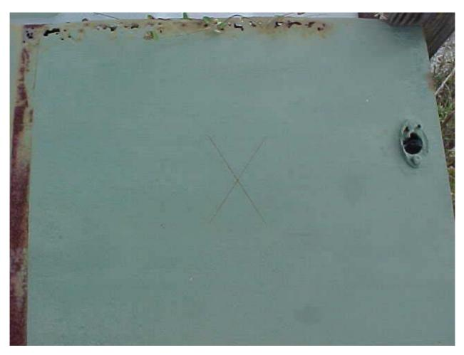
Quad Tests- This is closer picture of Upper Right Quad which is ZINGA Primer with CARC top coating- NO RUST present except Slight rusting at CUT where ZINGA is NOT present.
