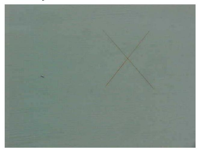
Quad Tests- This is closer picture of Upper Right Quad which is ZINGA Primer with CARC top coating- NO RUST present except Slight rusting at CUT where ZINGA has been removed by CUT
