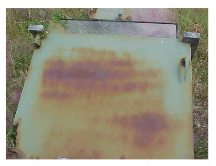
Control Door – typical epoxy paint used on truck door – 3 years of exposure in the sea side tests done by US Army
