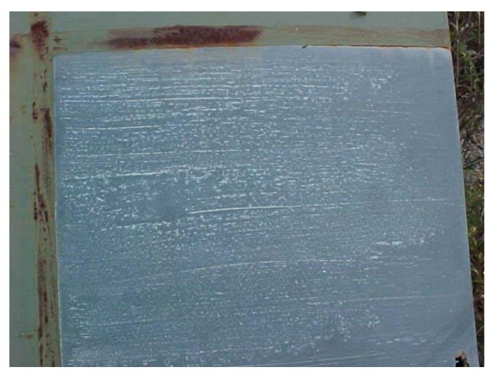
Quad Tests: This shows the Lower Right quadrant which was 'coated with ZINGA ONLY. The cathodic reaction can be seen clearly from the Zinc Salts (white-grey) forming on the surface. This shows SUPERIOR cathodic protection. NO RUST
